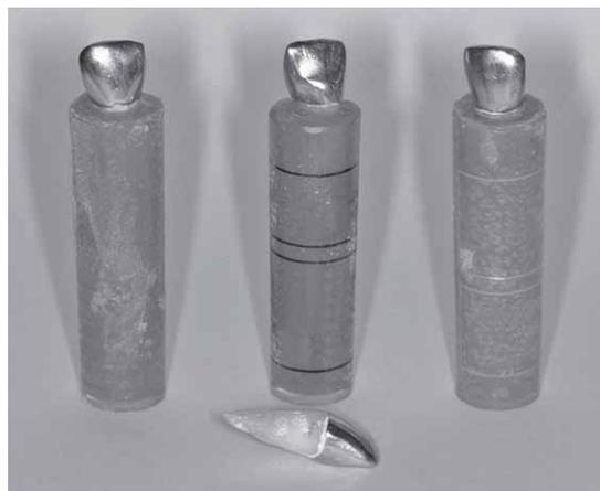
Fig. 2. Specimens with metal cast crowns embedded in acrylic resin.
