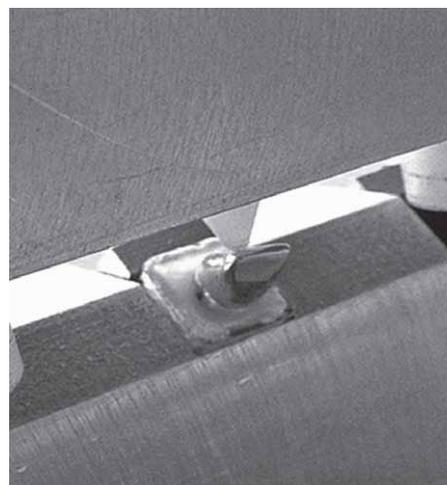
Fig. 3. Cyclic loading in the testing machine, with the load applied at the palatal surface.
