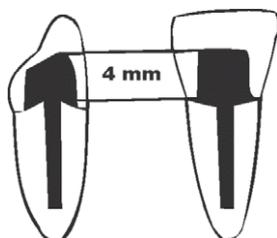
Fig. 1. Preparation of specimens with central parts of the palatal surfaces cut at an angle of 130°, 2 mm from the margins of the core.
